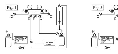
**NOTE:** Solution Indicates stop tap or valve - fit these whenever a hose has to be removed
