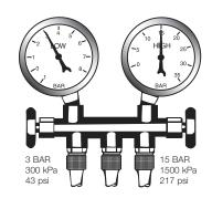
Compressor control valve malfunctionNote:Refer to workshop manual(Harrison V5 variable stroke compressor)for low side control point pressure
